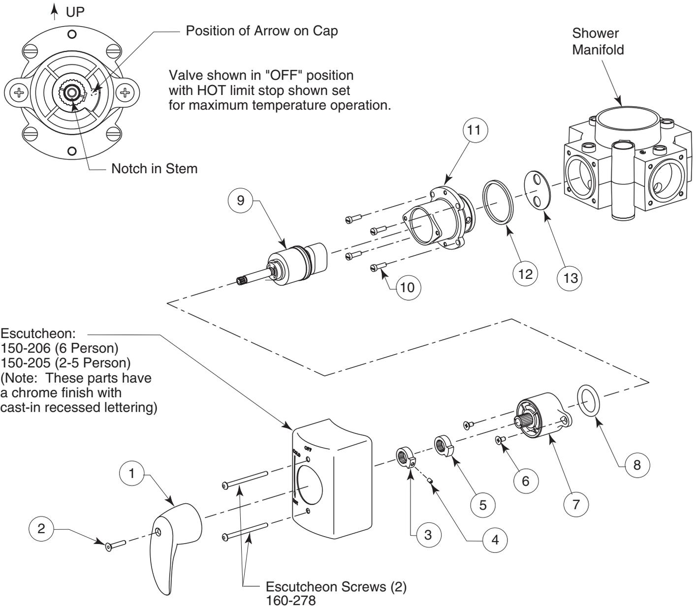
Equa-Flo valves are equipped with a temperature limit stop which can be used to limit the temperature of tempered water discharged.
